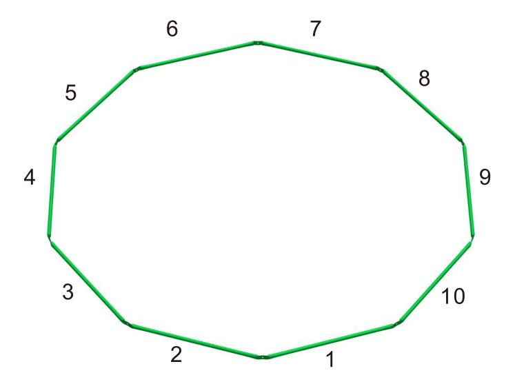
Slide an M8 Washer(#H) over  $\phi$  10 x 25mm Bolt(#F), then slide the Bolt(#F) through the joint of 2pcs Green Tubes(#A) on the ground, 1pc Yellow Tube(#B) and 1pc Green Left Gate Tube(#N) in the order indicated by the numbers. Slide another M8 Washer(#H) over the Bolt(#F) and secure with an M8 Nylon Nut(#G).
