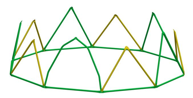
**Note:** Each joint at the bottom circle is connected by 4 tubes.
