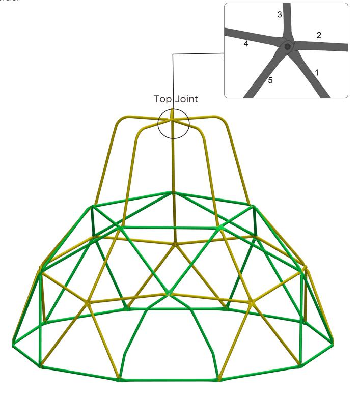
Install the Climbing Grips(#C) with M8 x 25mm Nut(#D) to cover the the bolt on each of the joint (except the bottom joints touching the ground), but don't forget the joint on the top.
