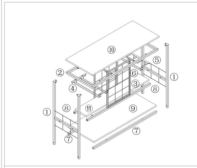
NOTED:Pls do not tighten all bolts until the products is assembled completely.
