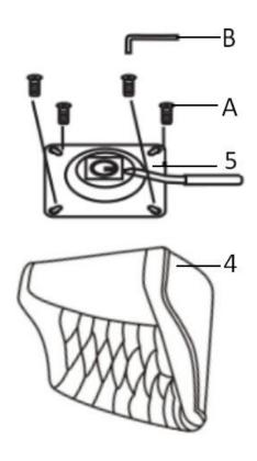
Attach bracket w/handle (5) to seat (4) by using bolt (A) and wrench (B) as shown.
