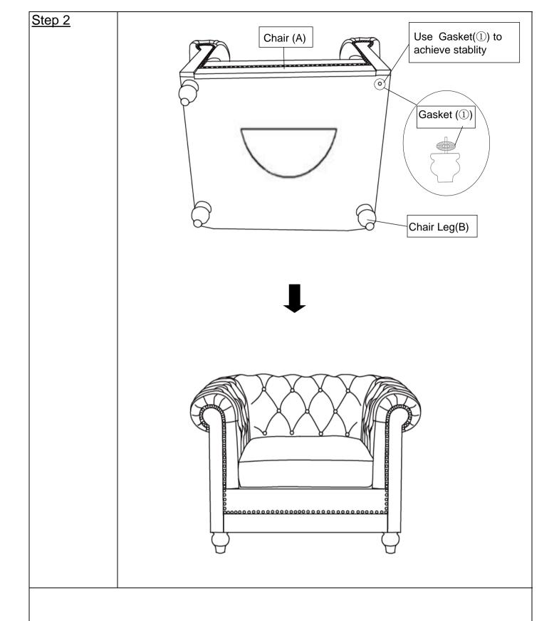
Install the Chair Leg(B) at the bottom of the Chair(A) by placing one  $Gasket(\mathfrak{D})$  on the threaded stem.
