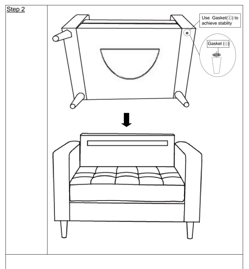
Install one of the Leg(D) at the bottom of the Chair(A) by placing one Gasket(①) on the threaded stem. Then insert the threaded stem into the threaded mounting position at a corner of the Chair(A).
