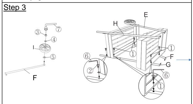
Repeat Step 1 to assemble the Wheel(I) to the Front Left Wheel Support(F). Then, align the Support(F)(G) to the Top and Bottom Shelf(A)(B) as shown above, using Bolts( $\mathfrak{D}$ )( $\mathfrak{D}$ )and the Allen Wrench( $\mathfrak{D}$ ).
