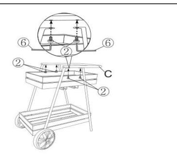
Position the Handrail(C) to the Supports as shown above. Attach the Handrail(C) to the Supports using Bolts(②) and the Allen Wrench(⑤).
