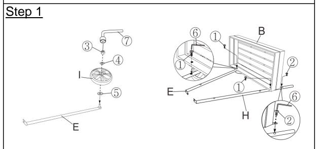
Place the Front Right Wheel Support(E) onto a clean, non-marring surface. Attach the Wheel(I) to the Support(E) using a Washer (4)(5) and Nut(3) with the Allen Wrench(7), tighten the Nut.
