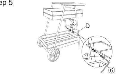
Take out the Middle Rack(D), and attach it using Bolts(②) and the Allen Wrench(⑤).
