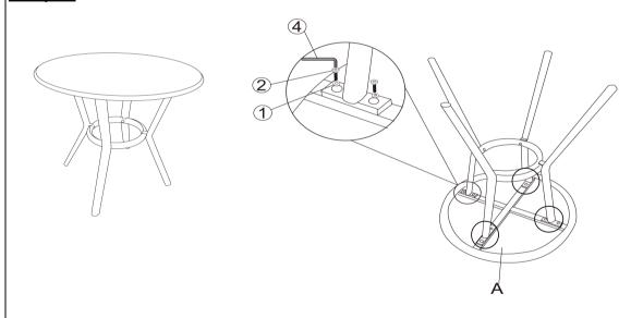
Attach one of the Legs(B) to the Table top (A) with the Bolts(2) and washers (1) using the Allen Key(4) as shown above.
