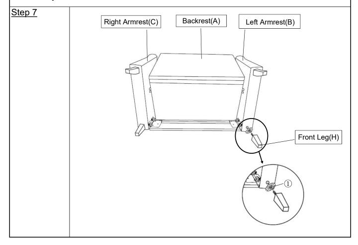
Install the Front Leg(H) to the Left Armrest(B) by using Plastic Washer(1) turning clockwise until tight. Repeat the same step with the remaining Front Leg(H).
