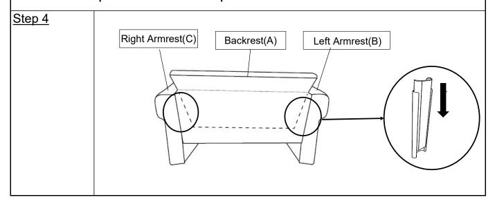
Slide the Tapered Connectors on the Backrest(A) into the Tapered Connectors on the Left Armrest(B) and the Right Armrest(C) as shown above.
