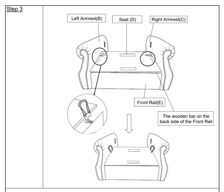
With the assistance of your adult partner, lift the rope on the two sides of Seat(D) by hand. Place the Seat(D) over the wooden bar on the back side of the Front Rail(E) and then slowly place it down on it as shown above.
