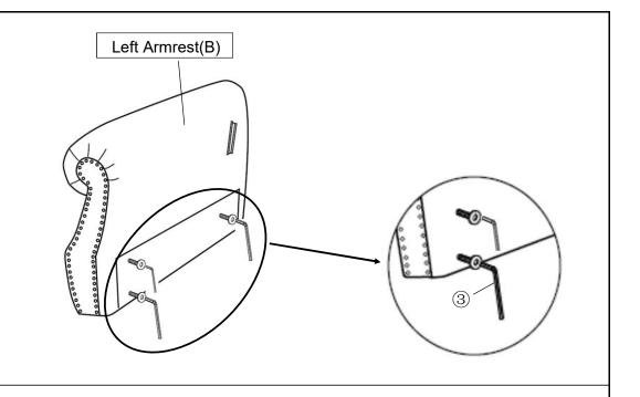
Open the carton and place all parts on a clean non-marring surface. Loosen the 3 bolts in Left Armrest(B) around half inch by Allen Wrench(③). Repeat the same step to loosen 3 bolts in Right Armrest(C).
