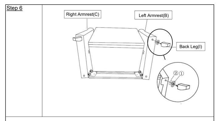
Install the Back Leg(I) to the Left Armrest(B) by using Plastic Washer(①) and Silicon Washer(②) turning clockwise until tight.
