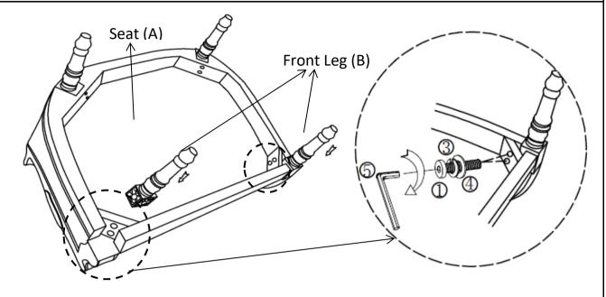
Attach the two Front Legs(B) into the mounting positions of the Seat(A) using Bolts(1), Spring Washers(3) and Washers(4) with the Allen Wrench(5). Do not fully tighten the Bolts.
