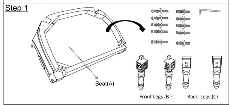
Place the Seat(A) on a clean, non-marring surface with the bottom facing you, as shown in picture above.
