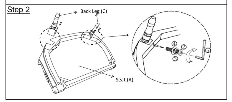
Attach the two Back Legs(C) to the bottom of the Seat(A) using Bolts(②), Spring Washers(③) and Washers(④) with the Allen Wrench(⑤). Do not fully tighten the Bolts.
