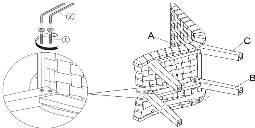
Turn the chair to the other side, then attach the Left Leg Panel (B) to the assembled part in step 2 by using the Bolts (1) with the Allen Key (2) as shown above.
