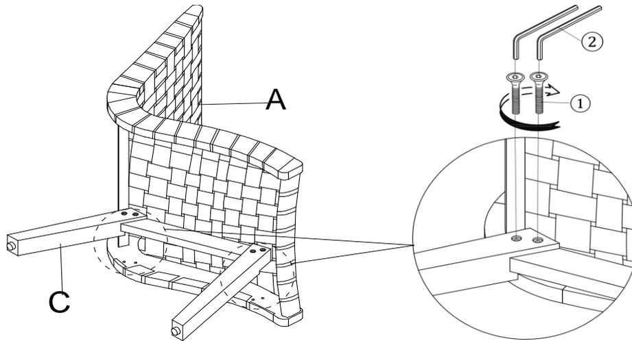
Place the Seat Panel (A) onto a clean, soft surface to avoid any scratches or damages to the product as shown in the picture above
