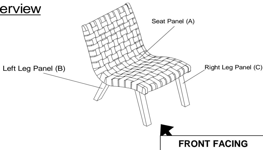
This Chair has multiple parts and may require up to 15 minutes to assemble. To give you an overview of the Chair parts, the above picture is provided to help you put the various parts into perspective. Please read through the instructions below to familiarize yourself with the parts and steps before assembly.
