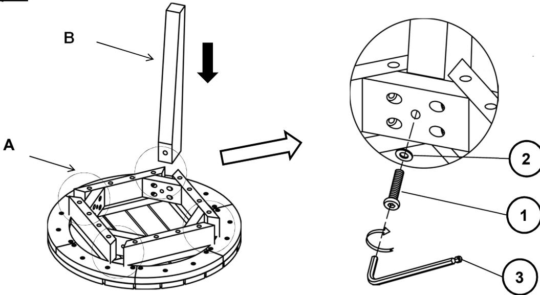
Attach Leg(B) to Table Top(A) using Bolts(①), and Washers(②) with Allen Wrench (③).
