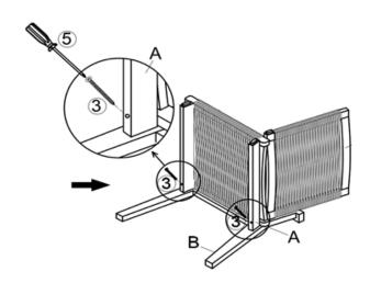
Position the Support bar (A) to the Left Leg Panel (B) as shown in the above picture.
