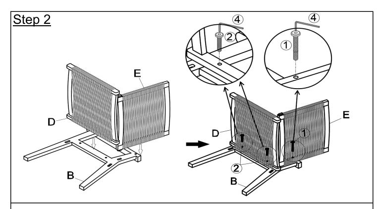
Position the Seat Panel (D) and Back Panel (E) to the Left Leg Panel (B) as shown in the above picture.
