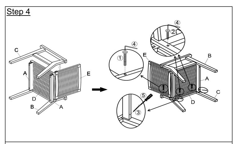
Position the Right Leg Panel (C) to the assembled parts in step 3 and turn the Chair into the opposite side as shown in the above picture.
