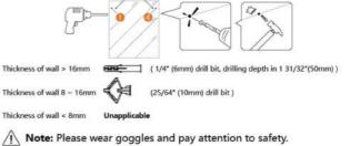
3. Screw the two brackets on wall.
