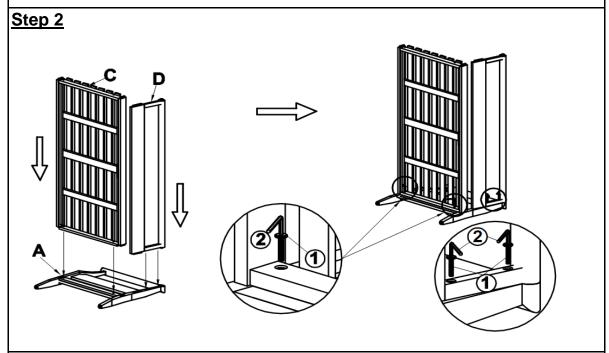
With assistance from your adult partner, position the Seat Panel(C) and the Backrest Panel(D) to the Left Leg Panel (A) as shown in the above picture. Then secure the Seat Panel(C) to the Left Leg Panel (A) using 2 Bolts( $\widehat{\ \ }$ ) and the Allen Wrench( $\widehat{\ \ }$ ).
