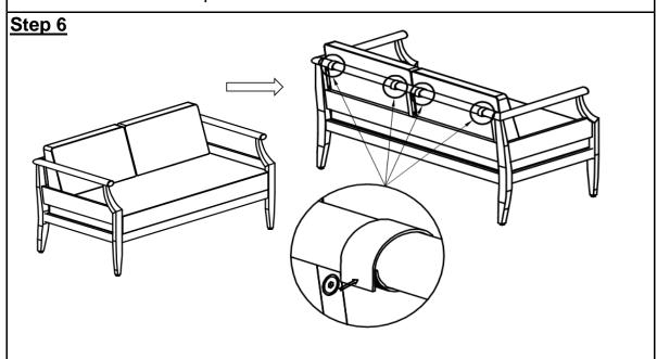
Tie the magic tape straps of the Back Cushion(E) and the Seat Cushion(F) to the Backrest Panel(D) and the Seat Panel(C) as shown in the above picture. Your Loveseat is ready for use.
