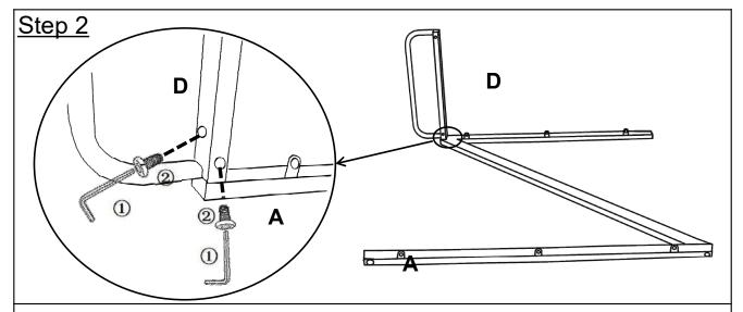
Attach one of the Handle (D) to the Right Frame(A) using Bolt(②) with the Allen Wrench(①).
