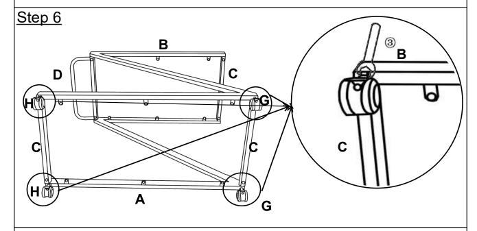
Attach the Wheels(G) and the Wheels with Brakes(H) to the Right Frame(A) and the Left frame(B) using the Spanner(③).
