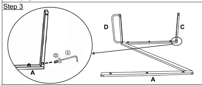
Attach one of the Support bar (C) to the Right Frame(A) using Bolt((2)) with the Allen Wrench((1)).
