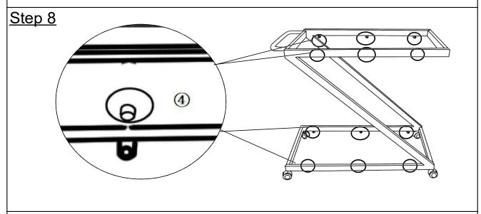
Attach the Glass Suction Cups (④) to the Pre-assembled Frame as shown.
