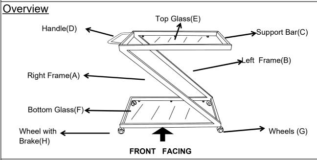
This Bar Cart has multiple parts and may require up to some 30 minutes to assemble. To give you an overview of the Bar Cart parts, the above picture is to help you put the various parts into perspective. Please read through the instructions herebelow to familiarise yourself with the parts and steps before assembly.
