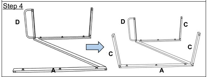
Repeat Step 2 to assemble the remaining Support Bars (C) using Bolts(2) with the Allen Wrench(1).
