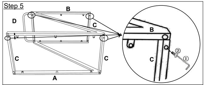
Repeat Step 1-4 to Connect the Left Frame(B) to the Pre-assembled Frame(A, C, D), using Bolts(2), with the Allen Wrench(1) as shown in the above picture. Note: Use your hand to straighten the bars and the handle of the Bar cart If you find that the screw hole position is uneven. Tighten the Bolts.
