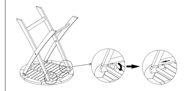
There are Wooden Locks, when the leg frame is in the correct position, rotate the Wooden Locks 90 degrees as pictured above.
