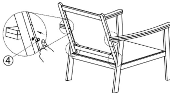
Cover the Bolts with Caps(4) after tightening.
