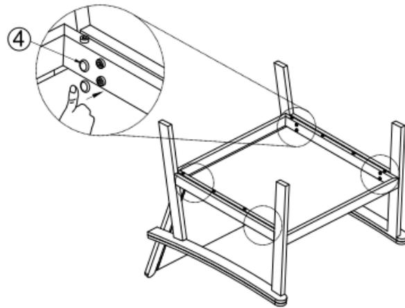
Cover the Bolts with Caps(4) after tightening.
