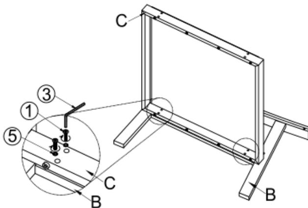
Attach Seat Panel (C) to Left Armrest (B) using Bolts (①) and Washers (⑤) with Allen Key (③).
