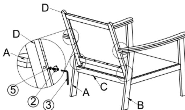
Attach Backrest(D) to Left Armrest(B) and Right Armrest(A) using Bolts(②) and Washers(⑤) with Allen Key(③).
