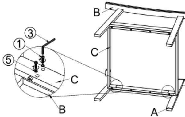
Attach Seat Panel(C) to Right Armrest(A) using Bolts(①) and Washers(⑤) with Allen Key(③).
