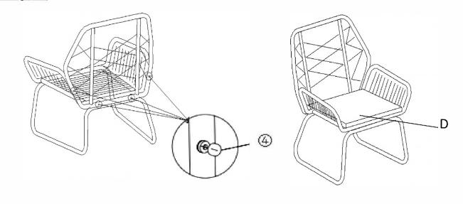
Put the PE Cap(4) on the bolts as the picture show above.
