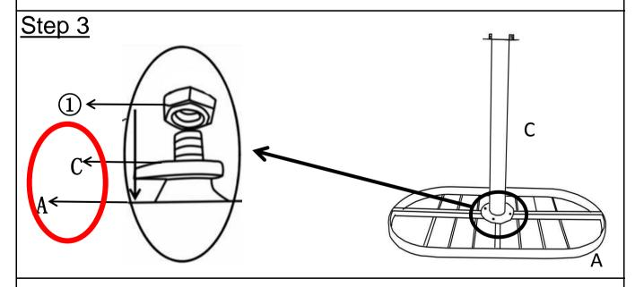
Attach the Support Ring(C) to Table Top(A) using Nuts(1) with Spanner(2). **Do not fully tighten the Bolts.**
