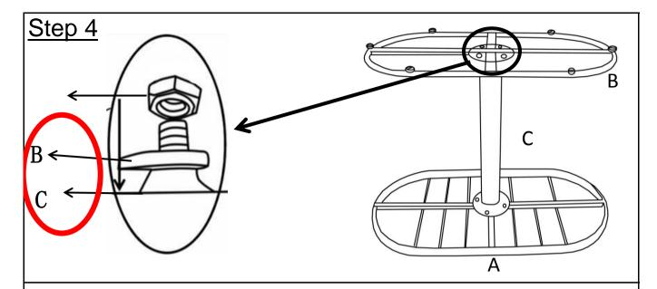
Attach the Support Ring(C) to Table Base(B) using Nuts( $\bigcirc$ ) with Spanner( $\bigcirc$ ). **Tighten all Nuts at all joints in a sequential manner.**
