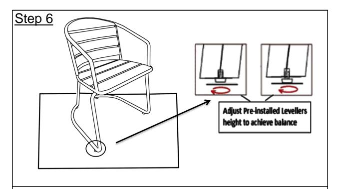
Adjust the Pre-installed Levellers at the base of the Legs until the Chair is level to the ground.
