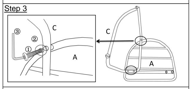
Align the mounting positions on Chair Leg(C) and Chair Seat(A), then attach using Bolts(1) and Washers(2) with Allen Key(3).
