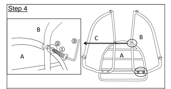
Align the mounting positions on Chair Leg(B) and Chair Seat(A), then attach using Bolts(1) and Washers(2) with Allen Key(3).
