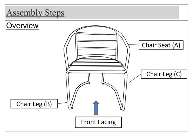
This Chair has multiple parts and may require up to 30 minutes or more to assemble. To give you an overview of the Chair, the above picture is to help you put the various parts into perspective. Please read through the instructions below to familiarise yourself with the parts and steps before assembly.
