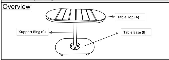
This Table has multiple parts and may require up to 20 minutes to assemble. To give you an overview of the Table parts, the above picture is to help you put the various parts into perspective. Please read through the instructions below to familiarise the parts and steps before assembly.
