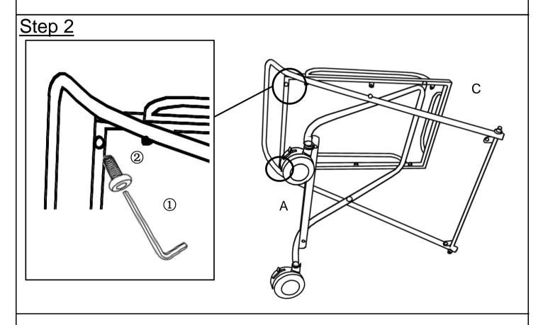
Attach Top Shelf(C) to Iron Frame(A) using Bolts(②) with Allen Key(1). **Do not fully tighten the Bolts.**
