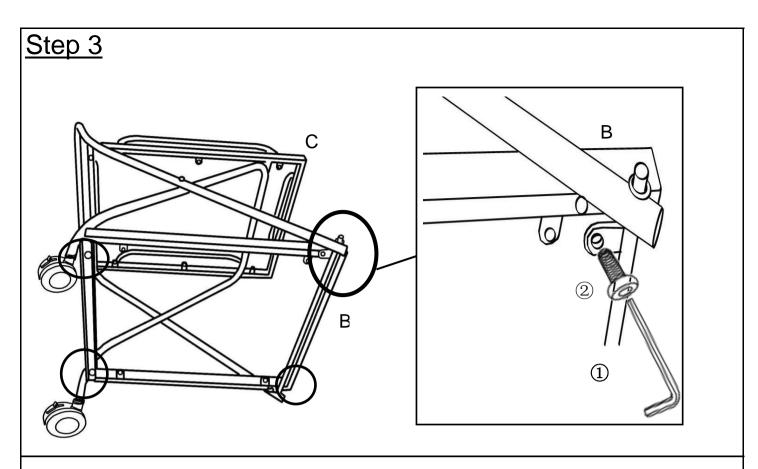
Attach Bottom Shelf(B) to Iron Frame(A) using Bolts(②) with Allen Key(1). **Do not fully tighten the Bolts.**
