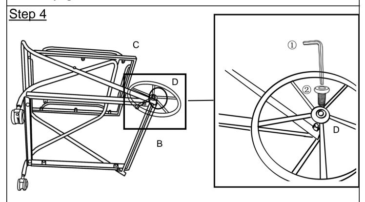
Attach Wheels(D) to Iron frame(A) using Bolts(2) with Allen Key(1).
