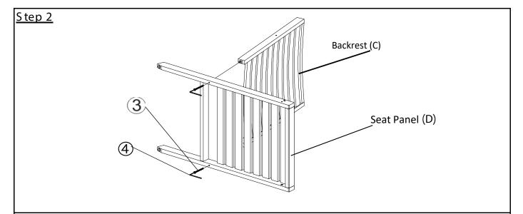
Attach Back rest (C) with the Seat panel (D) as shown in picture.
