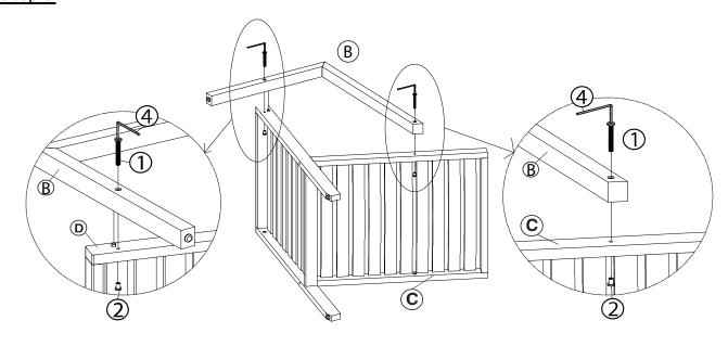
Attach Right Armrest (B) with the assembled frame in step 2 as shown in picture. Then secure the Right Armrest (B) with the assembled frame by using Bolts (1), Sleeve nut (2) and
