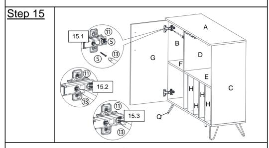
**15.1)** Attach the Connectors((11)) to the Left Side Panel (B) using Screws((5)) and a Screwdriver((13)).
