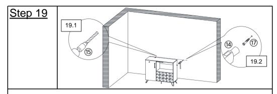
**19.1)** Using a Power Drill((15)),Drill two holes into the wall at the same height as Metal Brackets((16)) that you have placed on the Wine Cabinet.
