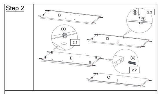
**2.1)** Insert Cam Locks(①) into the mounting positions on the Left Side Panel (B), the Right Side Panel (C), the Center Panel (D) and the Middle Panel (E) by hand.
