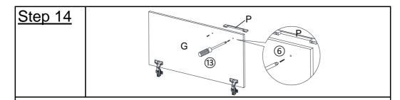
Attach the Handle (P) to the Door Panel (G) using Screws(6) and a Screwdriver(13).
