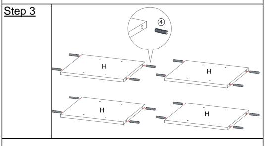
Insert Positioning Dowels(④) into the mounting positions on the Lower Spacer (H) by hand.
