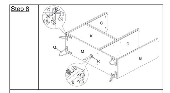
Attach the Legs (Q) and the Center Leg (R) to the Bottom Panel (M) using Screws(⑤) and a Screwdriver(①).
