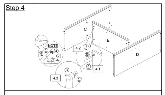
**4.1)** Insert the Positioning Dowels(④) of the Middle Panel (E) into the mounting positions on the Right Side Panel (C) and the Center Panel (D). Note: Ensure the arrows on the Cam Lock head points towards the Cam Bolt mounting position.
