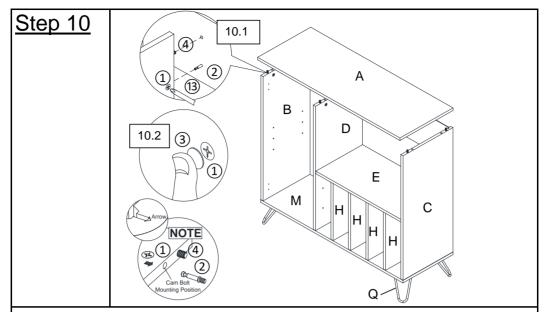
**10.1)** Insert the Positioning Dowels(④) of the Left Side Panel (B), the Right Side Panel (C) and the Center Panel (D) into the mounting positions in the Top Panel (A).
