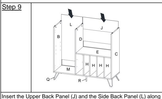
Insert the Upper Back Panel (J) and the Side Back Panel (L) along the slot on the Left Side Panel (B), the Right Side Panel (C) and the Center Panel (D).
