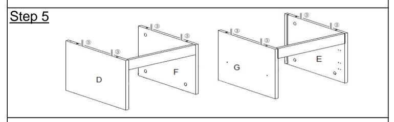
Insert Positioning Dowels(3) into mounting positions on Left Side Panel(D), Left Stand Panel(F), Right Stand Panel(G) and Right Side Panel(E) by hand as pictured above.
