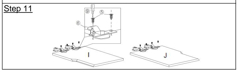
Attach Connectors(6) to the mounting positions on Left Door Panel(I) and Right Door Panel(J) using Screws(5) with Screwdriver(9) as pictured above.
