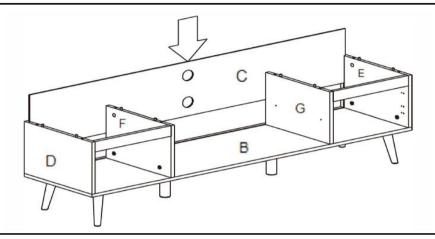
Insert the Back Panel(C) into the grooves on Left Side Panel(D), Right Side Panel(E) and Bottom Panel(B).
