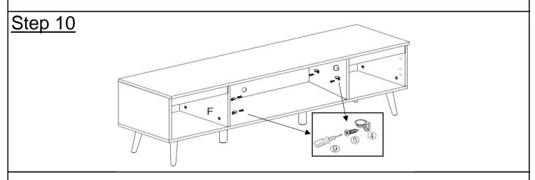
Attach Glass Clips(4) to Left Stand Panel(F) and Right Stand Panel(G) using Screws(5) with Screwdriver(9).
