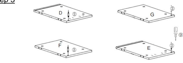
Attach Cam Bolts(②) to the mounting position on Left Side Panel(D), Left Stand Panel(F), Right Stand Panel(G) and Right Side Panel(E) using Screwdriver(⑨) as pictured.
