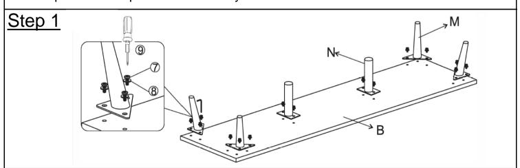
Take out all the Parts and Hardware, place them on a clean, non-marring surface. Place the Bottom Panel(B) facedown, then attach Legs(M) and Support Legs(N) to Bottom Panel(B) using Bolts(7) and Washers(8) with Screwdriver(9).
