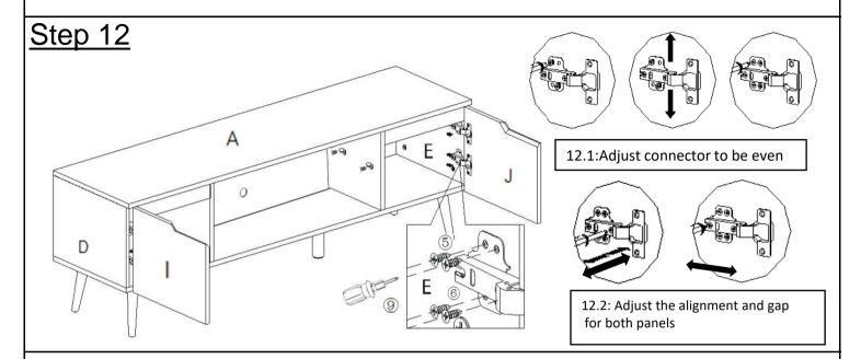
Attach Connectors(6) to Right Side Panel(E) and Left Side Panel(D) using Screws(5) with Screwdriver(9).
