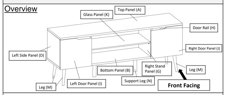
This TV Stand has multiple parts and may require up to 60 minutes to assemble. To give you an overview of the TV Stand parts, the above picture is to help you put the various parts into perspective. Please read through the instructions below to familiarise yourself with the parts and steps before assembly.
