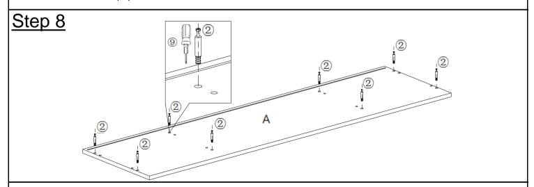
Attach Cam Bolts(②) to mounting positions on Top Panel(A) with Screwdriver(⑨) as pictured.
