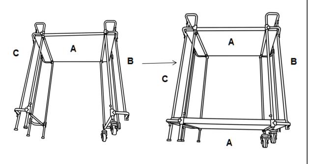
Attach bottom Wooden Tray(A) between Right Leg Frame(C) and Left Leg Frame(B) using Bolts(③) with Allen Key(④).
