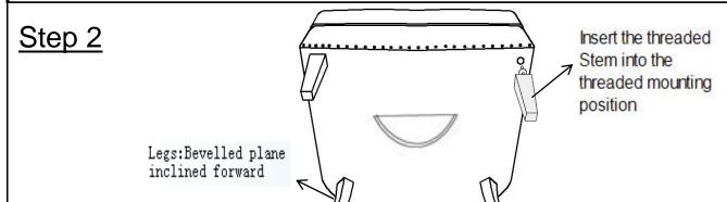
Install the first Front Leg(B) into the bottom of the Chair Base(A) by placing one Washer Ring(1) onto the threaded stem.
