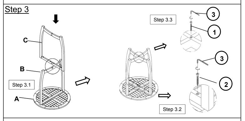
**3.1)** Position separated point of the Second Leg Panel (C) over the First Leg Panel (B) onto the Table Top (A).
