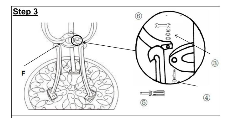
Attach the Leg Ring Support Ring(F)to Table Legs(E) using Bolts(4), Washers, Spring Washers, and Nuts (3).
