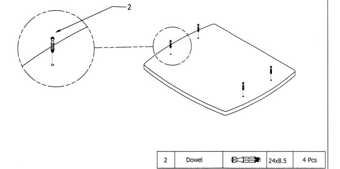
Step 4: Ready the cabinet structure and flip the Table Top (A) to cover on top of the cabinet. Then tighten the attachment with Ultra Shallow Cam (3) with Dowel installed in previous step 3. You would need to ready a screwdriver to perform this step.
